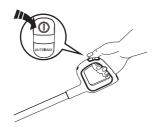
Press the button and the appliance will start in AUTO mode by default. Press it again to turn off the appliance. Switch between AUTO and MAX mode by pressing the AUTOMAX button.
