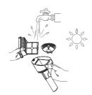
Grasp recessed area on each side of the HEPA and pull upward. Rinse under running water and must be completely dry before recombining with the lid of the DWT.
