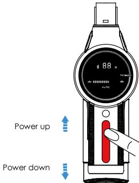
In AUTO mode, swipe the power control slider, and the appliance switches to Manual mode with "AUTO" indicator off.
